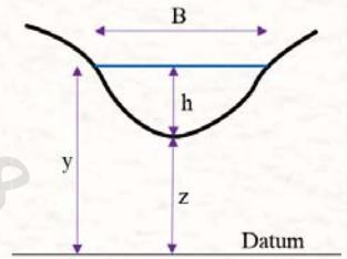
$$\begin{cases} \frac{\partial y}{\partial t} + \frac{A}{B} \frac{\partial u}{\partial x} + u \left( \frac{\partial y}{\partial x} + S_0 \right) + \frac{u}{B} \frac{\partial A}{\partial x} \Big|_{y=cte} = 0 \\ \frac{\partial u}{\partial t} + u \frac{\partial u}{\partial x} + g \frac{\partial y}{\partial x} + gS_f = 0 \end{cases}$$
