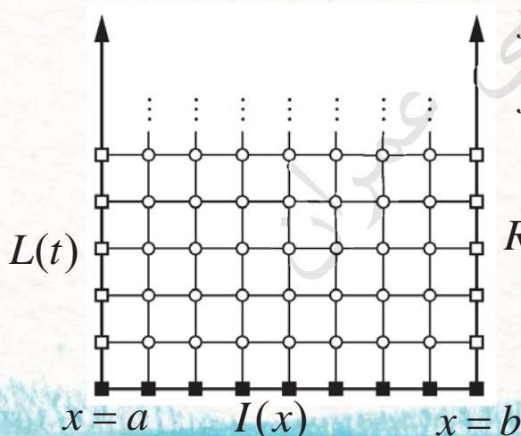
$$\begin{aligned} f(a, t) &= L(t) \\ f(b, t) &= R(t) \end{aligned}$$
