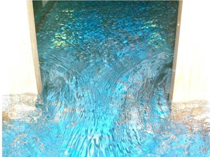
Figure 3. Flow at constriction with Discharge=15 lit/s and tail water =12 cm ( (view looking upstream).
